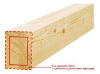
Figure 4: timber on the outside protects timber on the inside from fire
