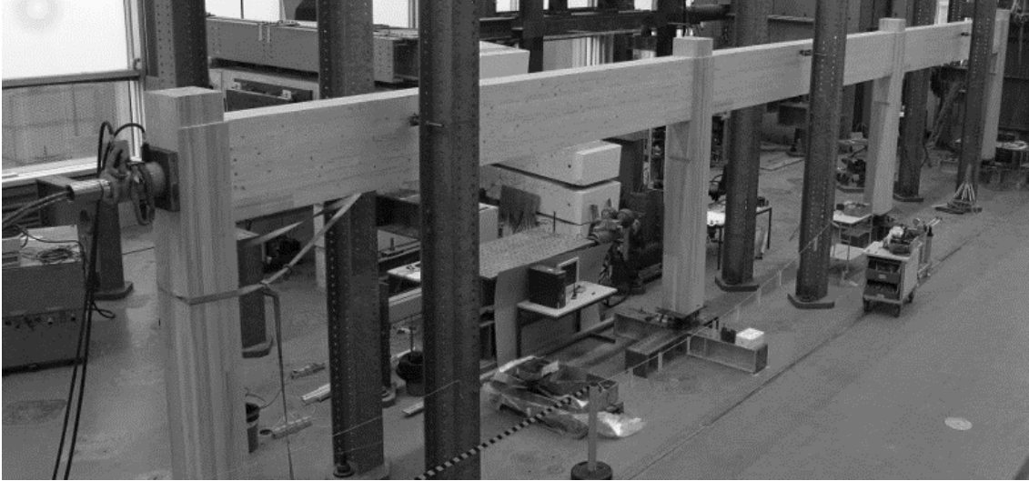
Figure 6: Test setup with a post-tensioned timber frame
