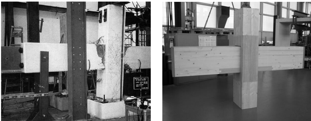
Figure 1: Post-tensioned concrete connection developed for the PRESSS-Program (left) [2] and the post-tensioned timber connection made of glulam developed at ETH Zurich [8]
